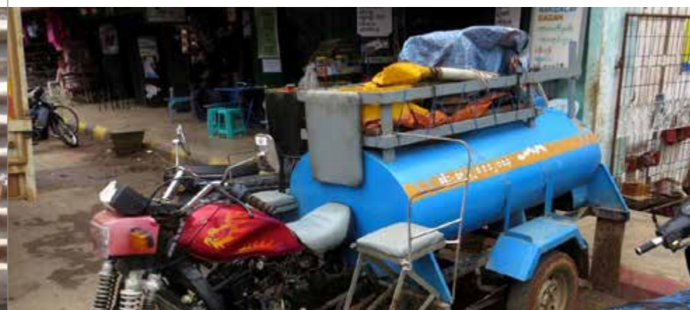
Mobile units to empty septic tanks
